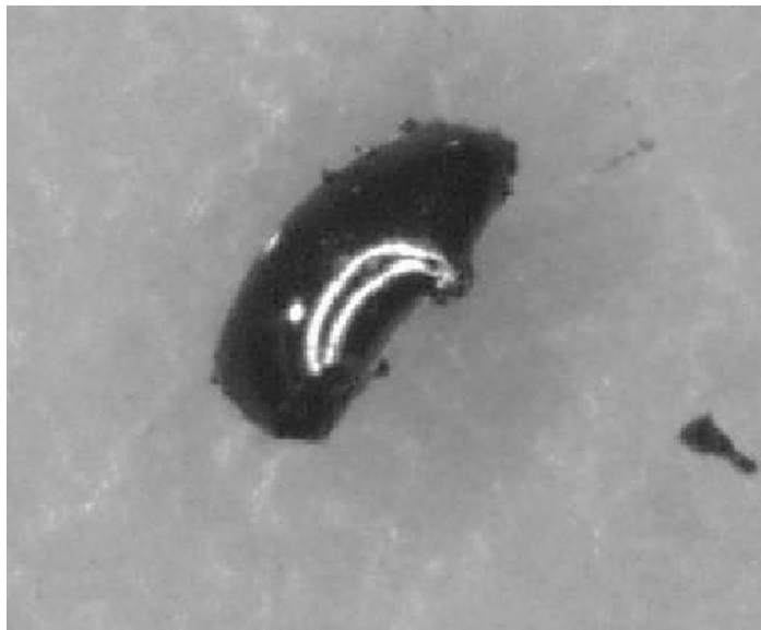
Figure 6. Optical image of sample showing the reflection of the light from the curved smooth top surface.
